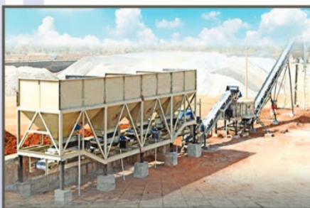
Wet Mix Mecadum Plant
