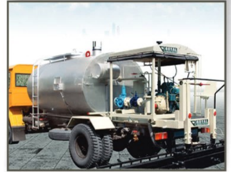
Bitumin Pressure Distributor
