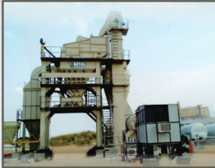
Batch Mix Plant (80/100/120/160 TPH)
